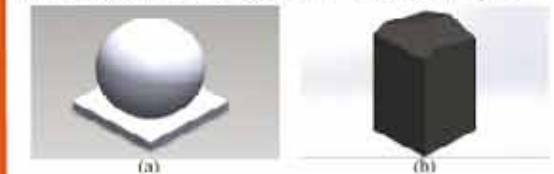
Figure.2: (a) isometric view of WBC attached to a rigid plate (b) isometric view of the berkovich indenter
